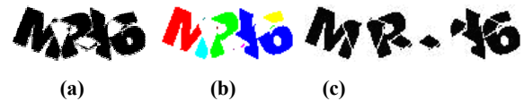
Figure 10. Failure when extracting black components. (a) original image, (b) a black component is shared by the last 2 characters as identified by color, (c) final segmentation output. Challenge reads “MRX6”.
