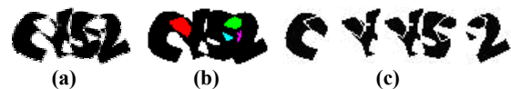
Figure 11. Failure of loop removal. (a) original image, (b) a lost connection area between the 2 nd and 3 rd characters, (c) final segmentation output. Challenge reads “CYS2”.
