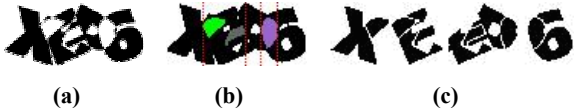
Figure 12. Failure of determining boundaries of shared white components. (a) original image, (b) failure to locate the connection area boundaries between the 1 st and 2 nd character and between the 2 nd and 3 rd character, (c) final segmentation output. Challenge reads “XEP6”.
