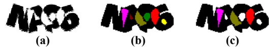
Figure 7. Identifying shared white components (a) original image, (b) after removing the image background, (c) after removing loops.
